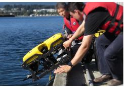
The **Chinook** is an industrial grade inspection ROV with a wide range of capabilities. Explore depths up to 300 m (1,000 ft) with the standard vehicle or 600 m (2,000 ft) with the deep water version.
