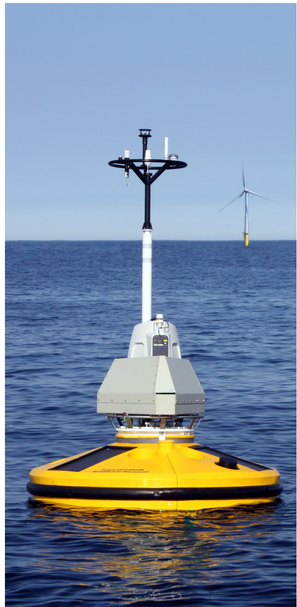
Accurate measurement of wind profile using SEAWATCH Wind LiDAR Buoy
