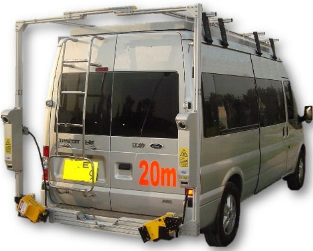
ROMDAS System with LRMS, Sub Meter GPS, High Resolution DMI and 2 Laser Profilometers.
