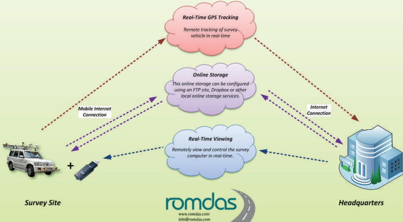
NB: The speed and quality of these services are dependant on local mobile internet speeds. Online Storage not recommended for systems using LCMS, LRMS or high resolution Video due to file sizes.
