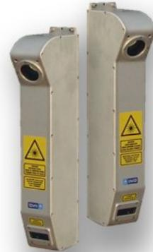
The TPL-LRMS can acquire full 4 m width profiles of a highway lane at normal traffic speeds. The system uses two laser profilers that digitize transverse sections of the pavement. Custom optics and high-power pulsed laser line projectors allow the system to operate in full daylight or in night-time conditions. LRMS also offers 2 sampling rate options; 30 or 250 Hz.
