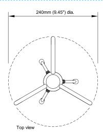
Positions for three off bolt fixings with 7.0mm (0.27") max. thread dia. on a p.c.d. of 85mm (3.35").
