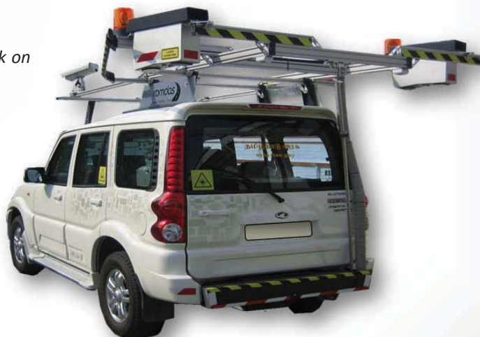
ROMDAS System with LCMS, Sub Meter GPS, High Resolution DMI, 3 Camera Video Module, Geometry Unit and 2 Laser Profilometers.
