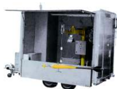
trailer with mechanical or electrical SEW - II for measurements from bridges
